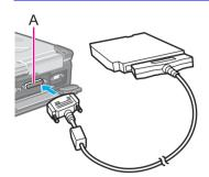
You may use the floppy disk drive as an external drive that is connected through the parallel port(A), by using an optional FDD cable (CF-VCF271).
