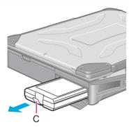
3 Pull the tab (C) on the battery pack and remove it from the computer.
