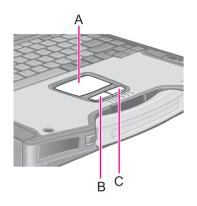
Use the touch pad to move the cursor on the display and perform normal computer operations.
