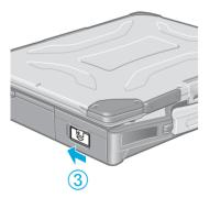
3 Lock the cover by sliding the latch to the left.
