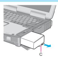
2 Pull the tab (C) on the hard disk drive and remove it from the computer.
