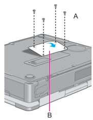
**3** Turn the computer over and remove the screws (A), then remove the cover (B).
