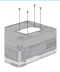
5 Put the cover back in place, then fasten the screws.
