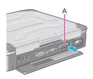
A printer can be connect to the parallel port (A) or the USB port ( page 70).
