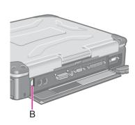
Connect the USB device to the USB port (A) or (B) on your computer, referring to the operating instructions of the USB device.
